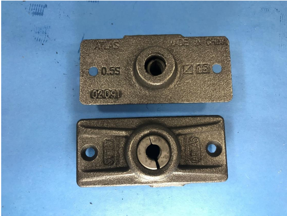
Figure 1. P.T. Atlas AN5S (0.5S) post tension anchor with a 1.2-in two-piece wedge
