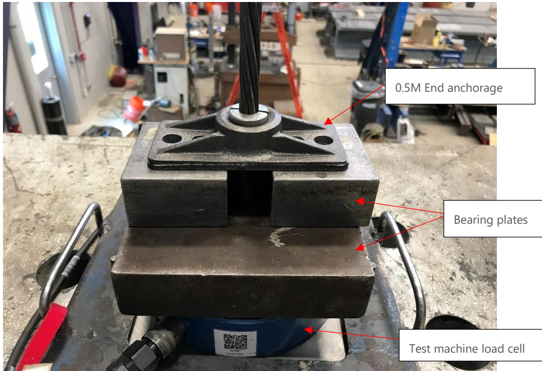
Figure 10. PTA 0.5M end anchorage bearing on test machine upper crosshead
