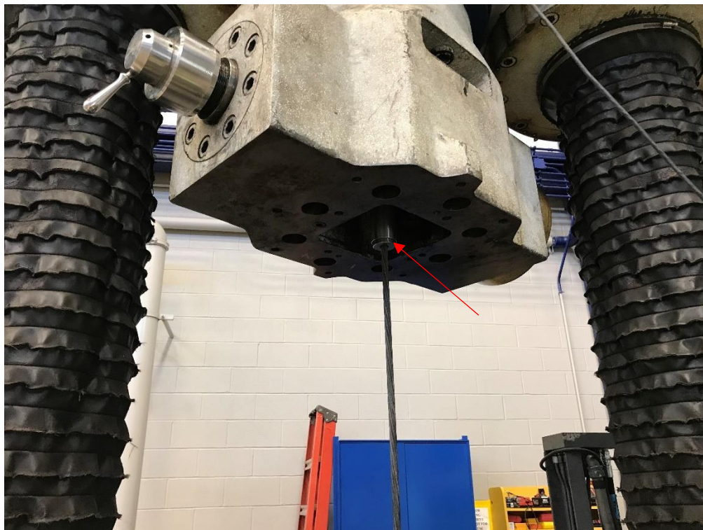
Figure 8. PTA SC500TU splice chuck at mid-length of test assembly
