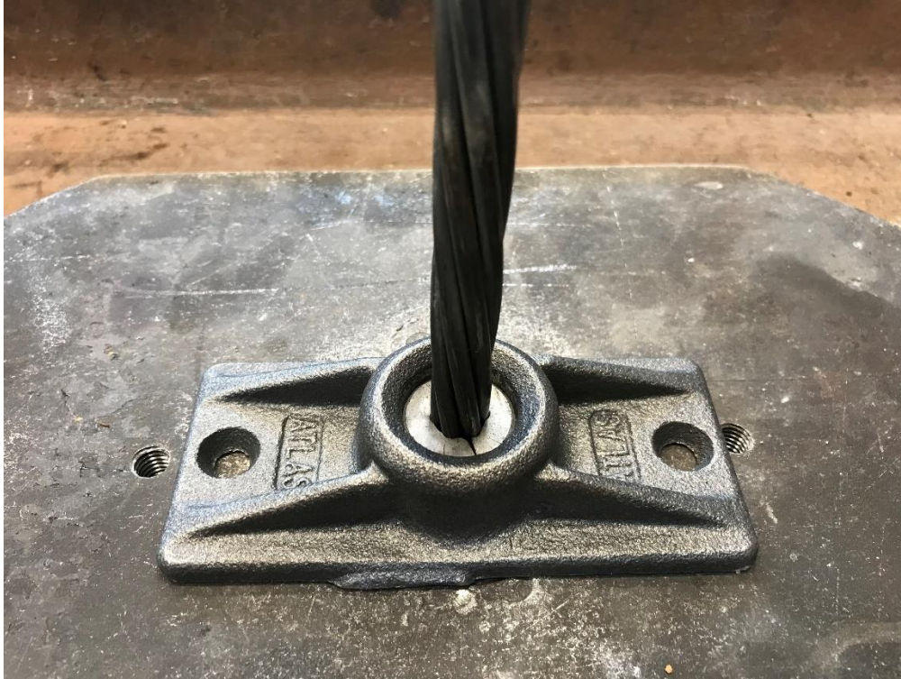
Figure 4. PTA 0.5S end anchorage at test machine top head
