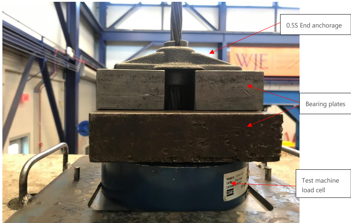
Figure 7. PTA 0.5S end anchorage bearing on test machine upper crosshead
