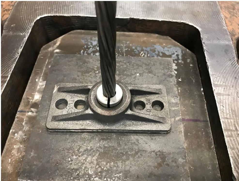
Figure 5. PTA 0.5M end anchorage at test machine top head
