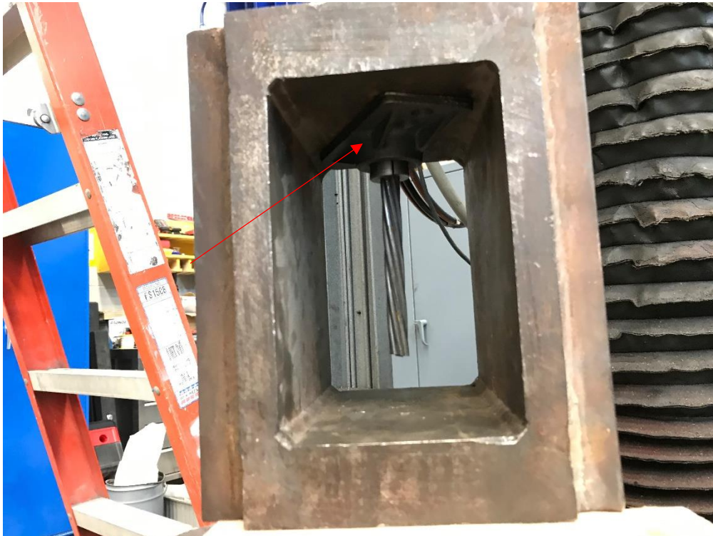
Figure 9. PTA 0.5M end anchorage in reinforced reaction fixture in test machine bottom grip
